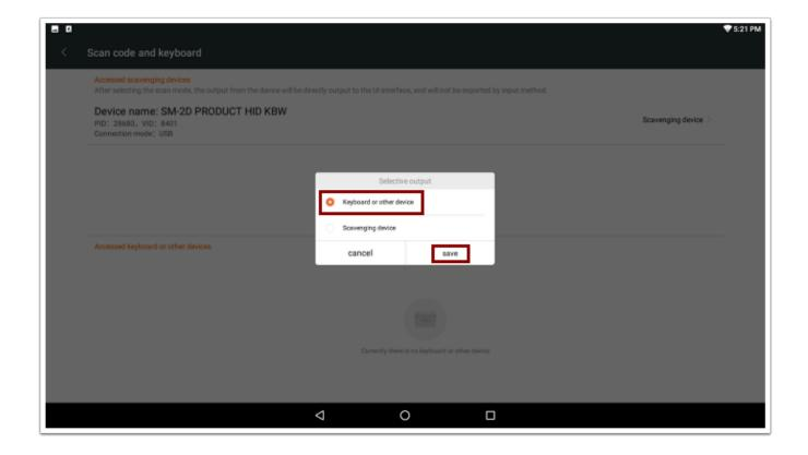
In order for the kiosk to properly recognize the scanner, it must be changed from a "keyboard or other device" to a "scavenging device," and then back to a "keyboard or other device."
