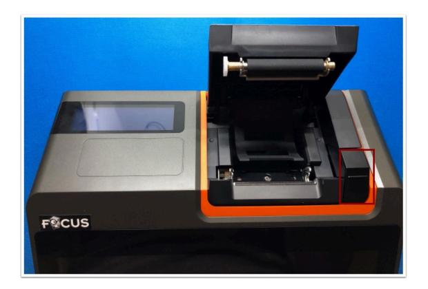
**2.** Insert the paper roll in the chamber, as shown.
