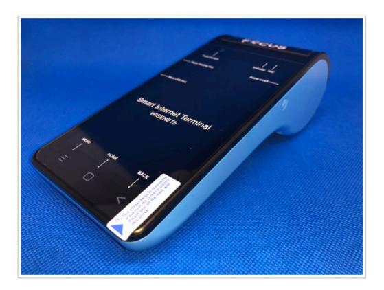
**2.** Turn on the handheld device by pressing and holding the power button on the right side for 3 seconds.
