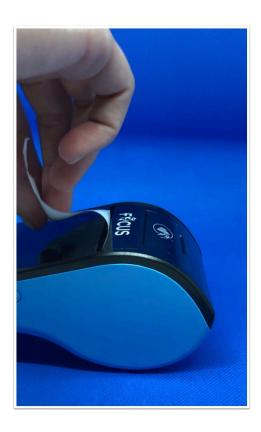
To feed the paper roll through the slot, press and hold the button on the left side of the handheld device.
